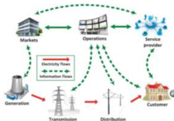
Fig1. Smart grid system architecture.
