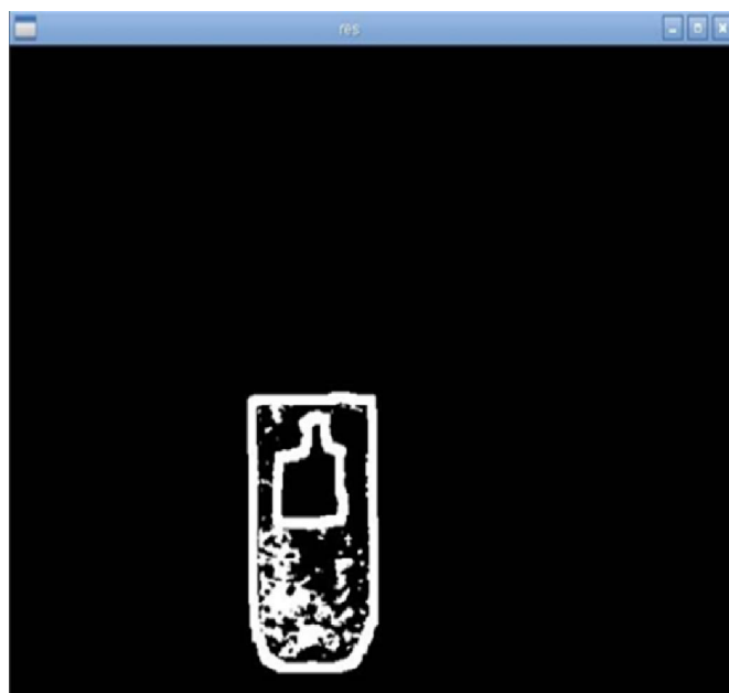
Fig. 12 hole filling and reference line matching
