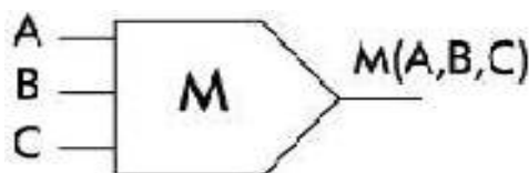
Fig 2: Structure of Majority gate
