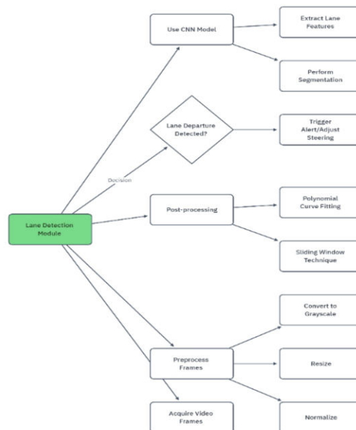
Fig 4.5.1: Data Flow of Lane Detection
