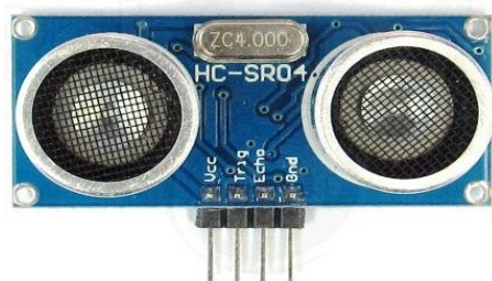
Fig 3. HC - SR04 ULTRASONIC MODULE:
