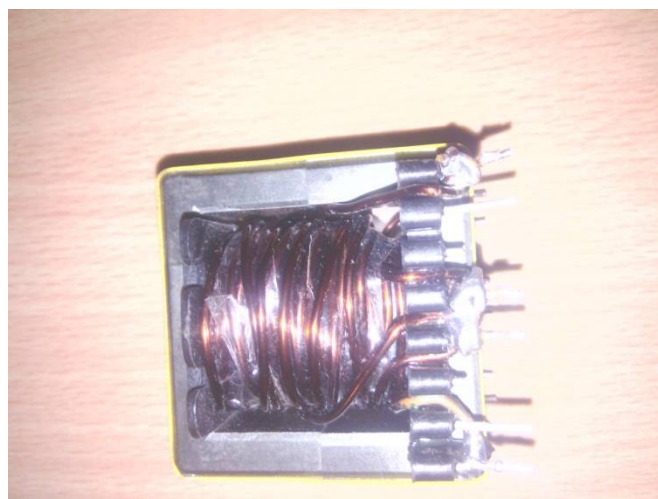
Fig.5. Winding of the transformer
