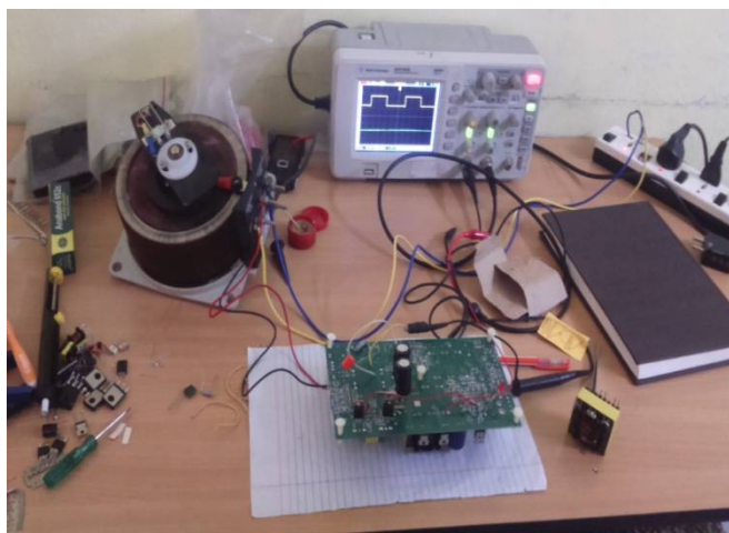
Fig.6. Hardware implementation setup of DC power supply
