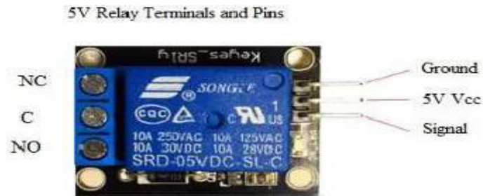
Fig 2. 5V Relay Terminal and Pins
