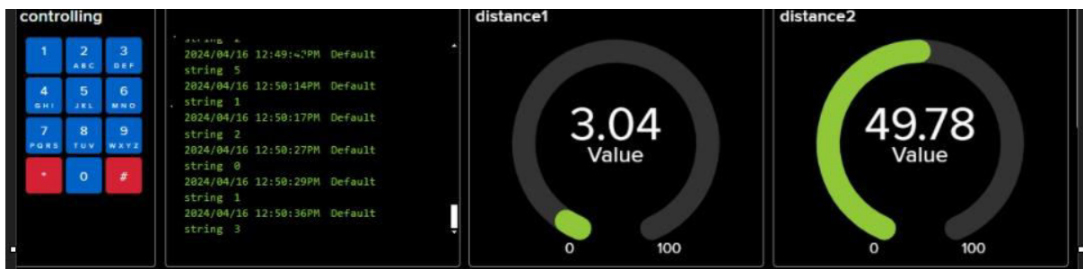
Fig 17. IOT Based Ouput of Distance 1 and Distance 2 (Ultra Sonic Sensor)
