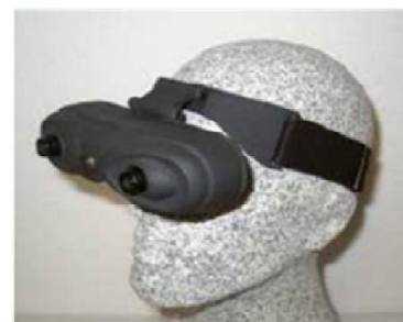
ARVision 3D HMD (commercial system) (cameras mounted over the eyes)
