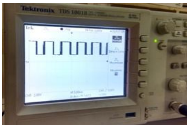
Fig.6 Waveform of Heart rate on DSO
