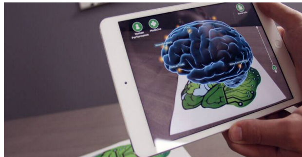
Figure 1: The user points a smartphone screen on the textbook and then augmentation is seen with more information on the screen. [6]
