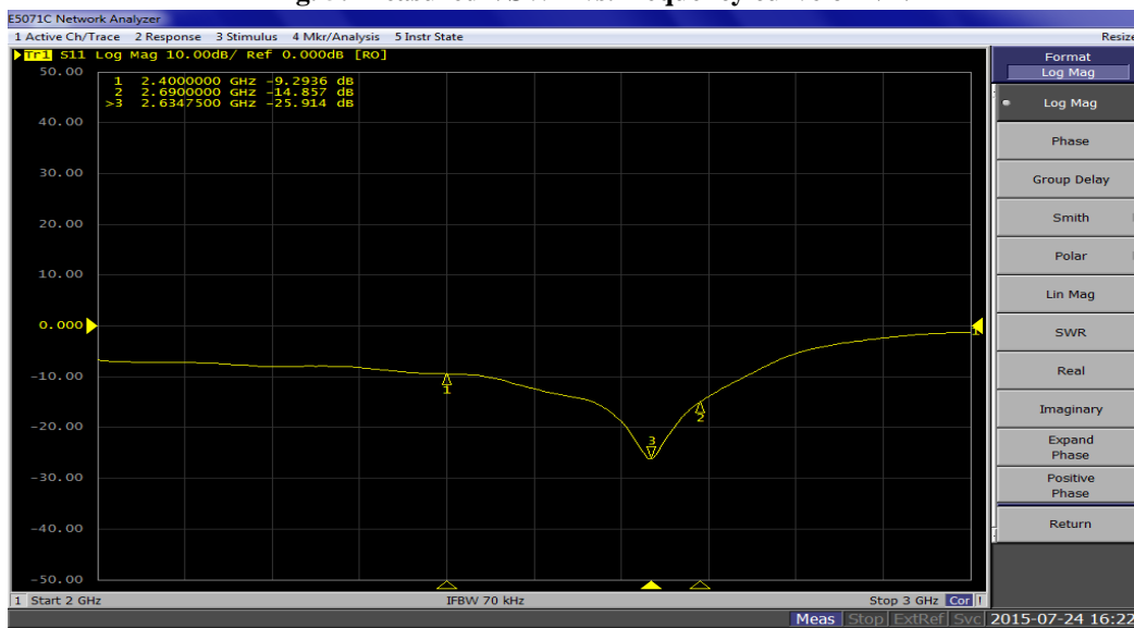
Fig. 6: Measured return loss vs. frequency curve on VNA
