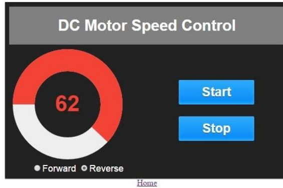
Fig.III. IoT Dashboard for DC Motor Speed Control
