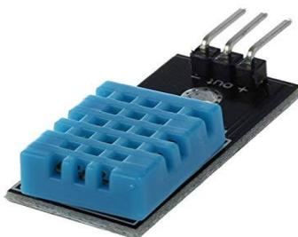
Fig 4: Temperature and humidity sensor
