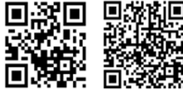
Fig. 1. Three different barcodes encoding the statement "Virtual reality". (a) is a linear barcode (code 128), and (b) and (c) are matrix barcodes (of the QR code standard). While (b) encodes the plain text, (c) encodes an encrypted version using the AES-256 encryption algorithm in the cipher-block chaining (CBC) mode (note this last code requires a password for decryption).
