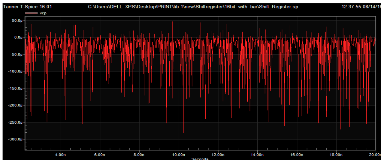
Chart 1. Power consumption graph of proposed 16 bit shift register.
