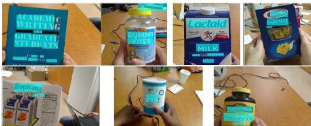
Fig:7. Some results of text localization on the user-captured dataset, where localized text regions are marked in blue.
