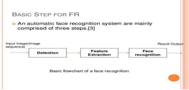
Fig 1.2 basic diagram of face recognitio
