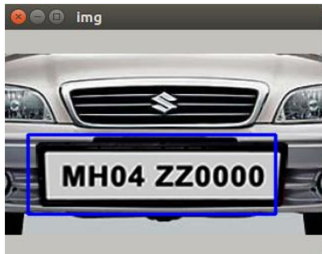
Fig 3. Plate Detected using HOG + SVM Classifier
