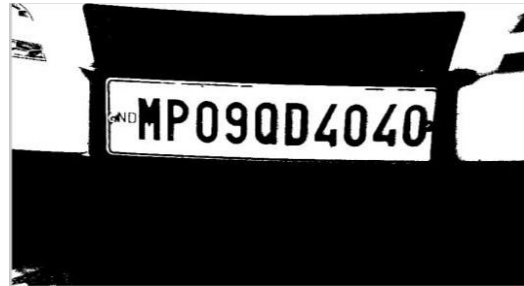
Figure 5; After Dilation, Erosion and converting it into Binary Image.
