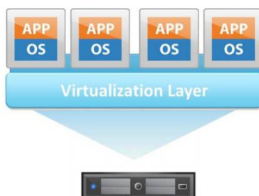
Fig.2. Descriptive image of Virtualization based on physical Operating System with CPU/Memory/Network Segregated Environment and Ecosystem thus forming the Infrastructure for Cloud Computing .
