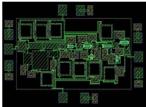
Fig.11. Layout of IC for LNA Design
