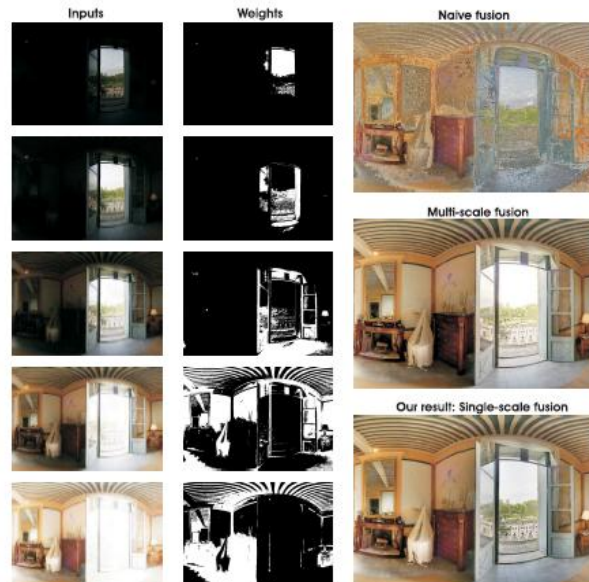
Fig.1. Naive, multi-scale fusion and our single-scale result. Both involve, a similar degree of complexity, while our single-scale fusion method is able to deliver results competitive with the multi-scale approach.
