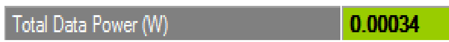
Fig.15. Power consumption of convolutional encoder and Parallel processed viterbi decoder with pipelining technique.
