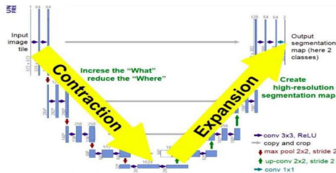
Fig 3. Contraction &Expansion process of the U-NET architecture by Olaf Ronneberger et. el.
