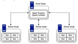
Fig. 5: Architecture of Apache Spark
