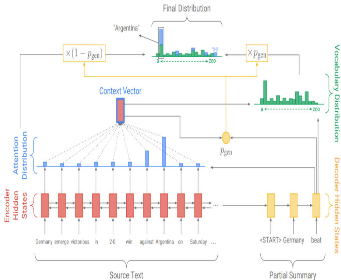
Fig 1: Architecture of Pointer-Generator Model
