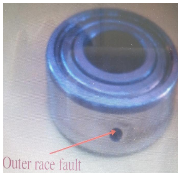
Fig. Outer race bearing fault
