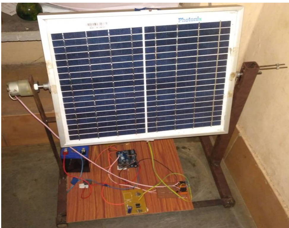
Fig.2. Solar PV developed with Sun tracking
