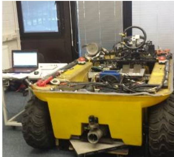
Fig. 1 water jet mounted on AAV (DORIS)
