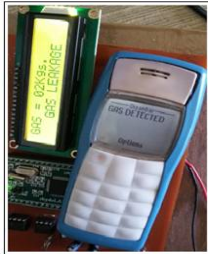
Fig. 2 Gas Leakage Detected
