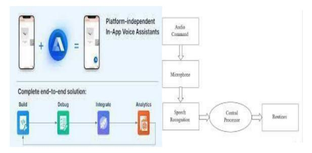
Speech is input into the speech recognition module, which converts it into signals. The central processor processes the transformed text and outputs the required result [2]. A few other installed modules and libraries, including Speech Recognition, Wikipedia, GTTS, date time, OS, pyaudio, requests, and a web browser, are also included in the system architecture[4].
