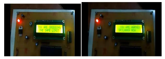
The boat distance can be measured using the received signal strength received from the slave RSSI (boat). Arduino UNO is used as the controller which controls the proposed system. By using this RSSI we can find the location (zone) of the boat in the sea. Whenever the boat is to reach the border the APR voice alert the concern person in the boat and at the same time boat will automatically turn OFF.LCD is used to print the current status from the controller.
