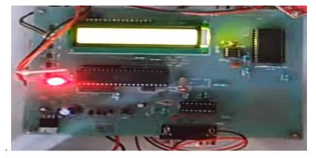
In this module implement the three zones, that is safety zone, intermediate zone and danger zone. Ultrasonic sensors are based on measuring the properties of sound waves with frequency above the human audible range. They are based on three physical principles: time of flight, the Doppler effect, and the attenuation of sound waves.
