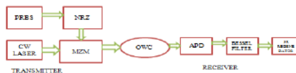
Figure: 5 Block diagram of 1TX/1RX IsOWC system.
