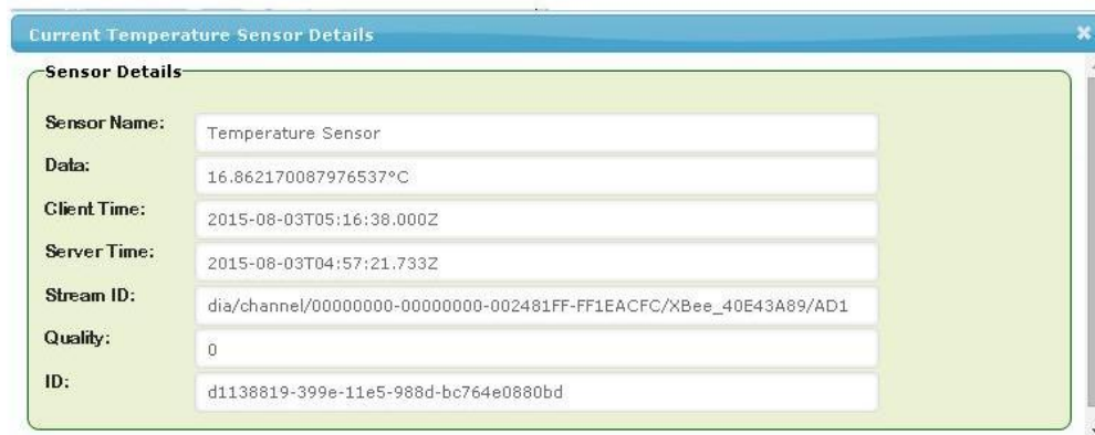
Fig. 6 The pop up window showing the temperature details (fetched from Digi cloud)
