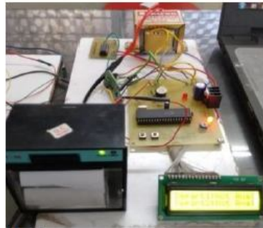
Fig : System of token generator using CC2500
