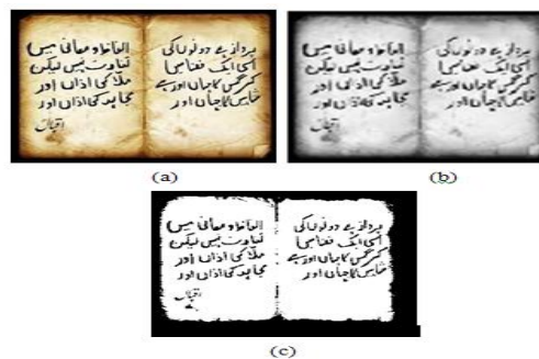
FIGURE II: Sample images obtained in different stages (a) input Image(b) Grayscale Image (c) Binarized Image
