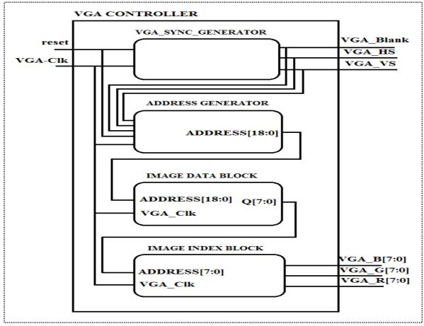
Fig.2. Internal Block Diagram Of VGA Controller.
