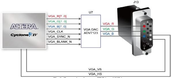
Fig 8. Connections between FPGA and VGA
