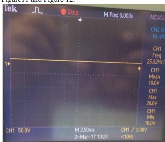
Figure 9: Secondary output voltage 1(Vout1) of 18V
