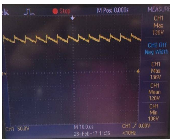
Figure 8: Reflecting Voltage across snubber circuit
