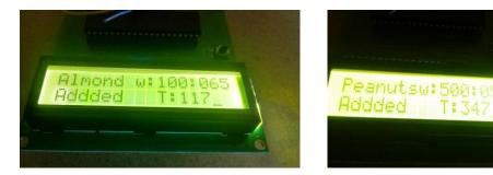
After completion of the shopping, press the shopping completed button. The image as shown below is seen and the information is sent to the PC using ZIGBEE technology.
