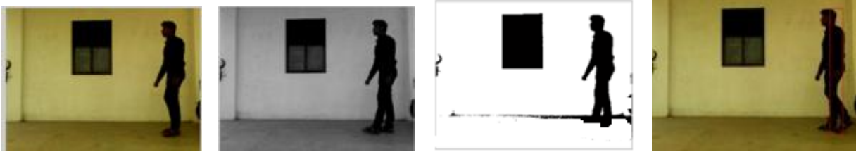
Figure : (1) Background Image (2) Original Colour Video (3) Gray Scale Image (4) threshold Image (5) Original Image with Bounding Box .
