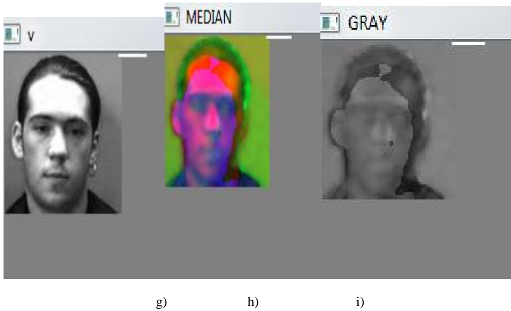
Fig 3.a)Original image b) Region of interest (ROI) c)Resized image d) color transformed image e) hue f) saturation g) value h) median filter i) gray image
