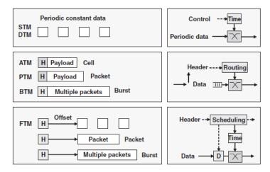
Figure 5.Different Switching Techniques
