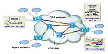
Figure 4.Optical Burst Switching Technique
