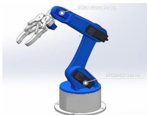
Figure1. Complete design of the robotic arm
