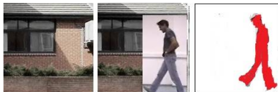
Fig.3. Adaptive Background Subtraction sample.(a) Predictable background (b) Recent image (c) Detected region
