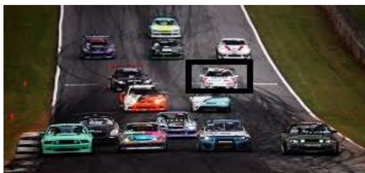
Fig. 1. Example of clutter in video. Target object (shown with black square) and other car in background are similar in colour.
