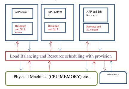
Fig. 1. The framework For resource allocator and Load Balancing.
