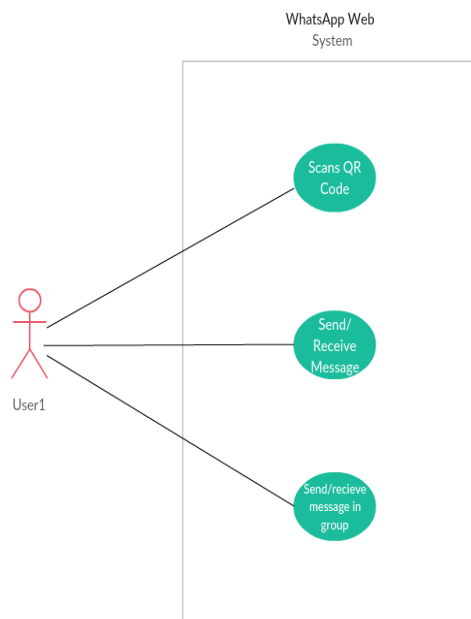
Fig IV. A2: WhatsApp web Use Case diagram
