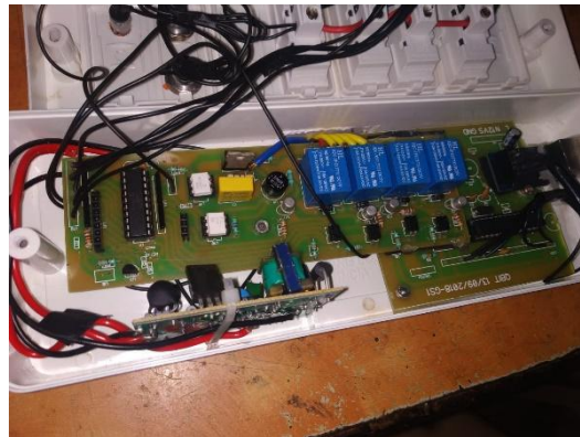
Fig(i):Kit Diagram for Home Automation[1]
