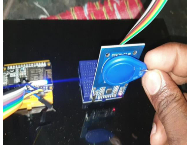
RFID reader reads the RFID Tag
